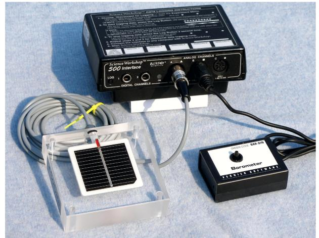
Connect the pyranometer to Science Workshop input A and the barometer to input B as shown. The serial cable is connected to the PC with the Science Workshop software installed. Connect power to the unit.
